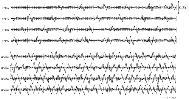
Fig. 4 Low-pass filtered pressure trace near rotor leading edge in flow range A
